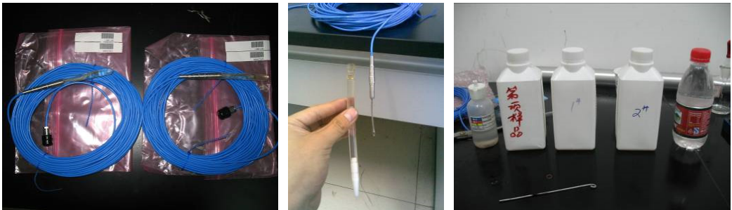
Fig. 2. Test two new ICP underwater shock wave sensors and five silicone oils
