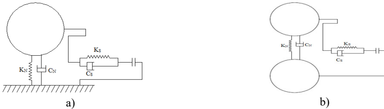
Fig. 1. a) Ball-wall spring mass diagram, b) ball-ball spring mass diagram
