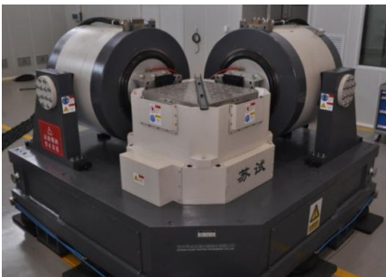
Fig. 3. Triaxial vibration test system
