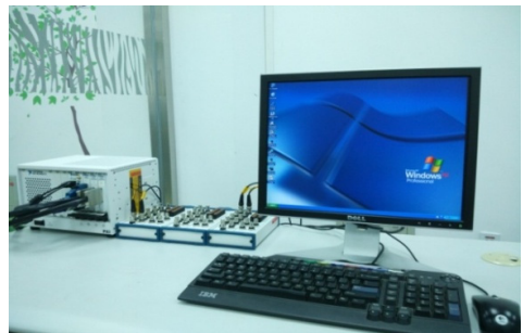
Fig. 4. Multi-axis sine vibration controller
