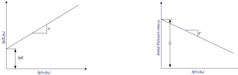
a) The relation between \lg(E_i/p_a) and \lg(\sigma_3/p_a) b) the relation between \mu_i and \lg(\sigma_3/p_a)
