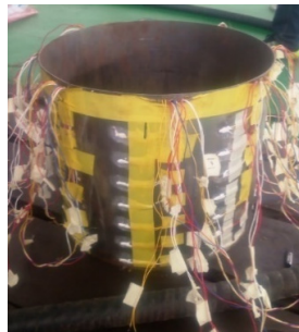
a) Overall view of the confined test device b) Strain gauges on outer surface of thin-walled bucket
