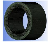
Fig. 2. FEM model of stator and winding
