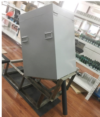
Fig. 4. The installation and debug of automatic launcher of XBT probes
