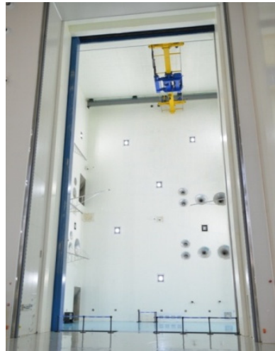
Fig. 6. 4000 m 3 acoustic chamber
