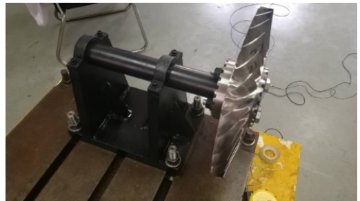
Fig. 4. Installation boundary condition test
