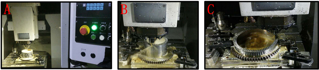
Fig. 6. Milling machining: a) of level 1 face gear sample, b) of level 2 face gear sample, c) of level 3 face gear sample
