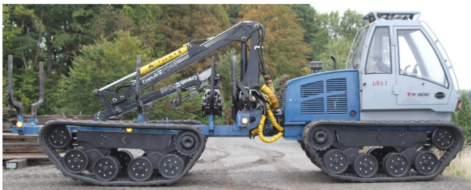
Fig. 1. Real prototype of forwarder with four tracked undercarriages (without the load) [3]
