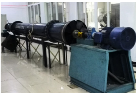
Fig. 4. Test bench of cooling fan
