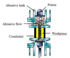
Fig. 1. Abrasive flow processing principle
