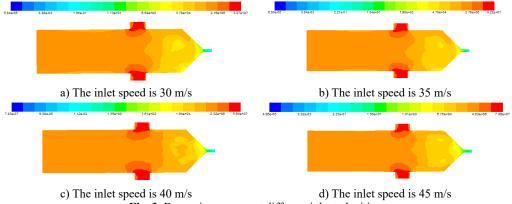
**Fig. 3.** Dynamic pressure at different inlet velocities
