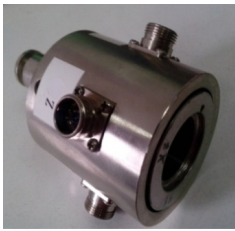
a) Trimming three-way force sensor
