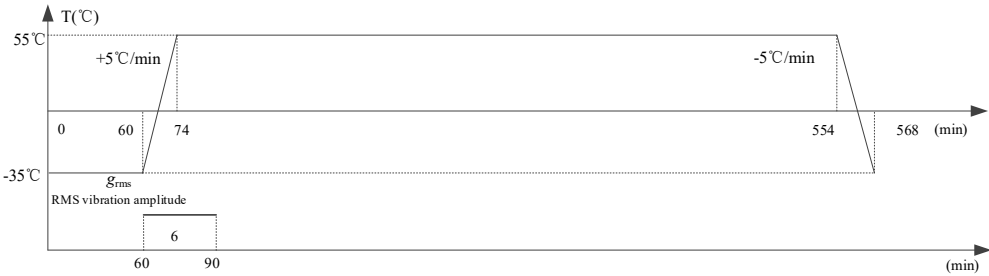
Fig. 2. Test profile of RQT for the equipment
