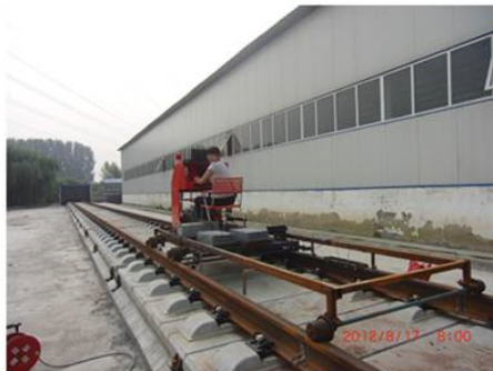
Fig. 1. The track fastener inspection vehicle
