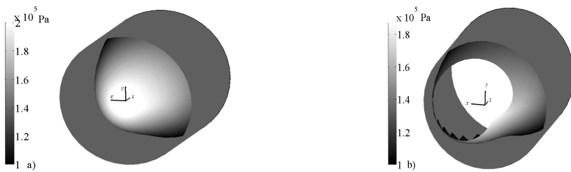
Fig. 3. Typical pressure profiles for lubricant supply without a) and with b) accounting Lomakin effect ( \omega = 314,16 rad/s, e = 0,4 , p|_{z=0} = 2 \cdot 10^5 Pa, p|_{z=L} = 1 \cdot 10^5 Pa)
