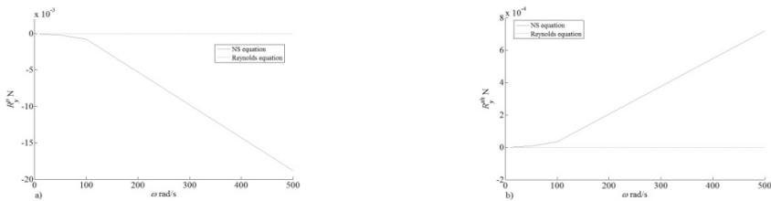
Fig. 5. Fluid film reaction ( \alpha = 0.001 ) component Y for pressure a) and for shear stress b)
