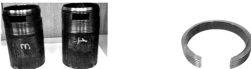
Fig. 7. Preparation of samples for microhardness testing using PMT-3 microhardness tester
