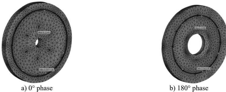
Fig. 3. Simulation of eigenfrequency of the circular waveguide
