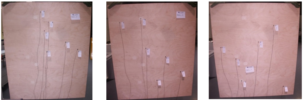
Fig. 1. Plywood panel with different accelerometer distributions
