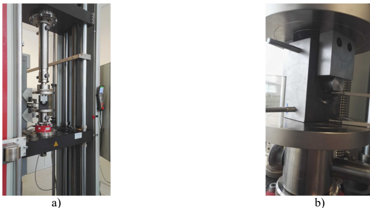
Fig. 2. Arrangement of technical experiment for a determination of static characteristic of a) rubber element and b) detail of test sample
