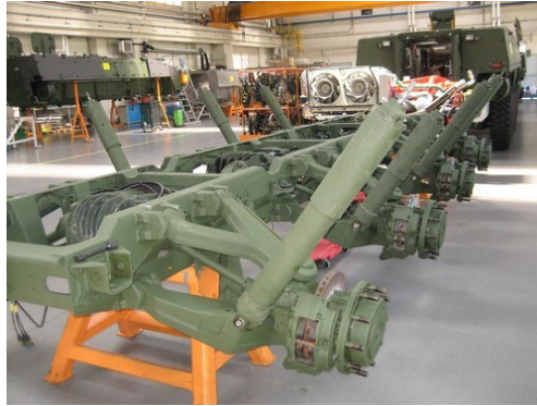
Fig. 4. Frame and hydro-pneumatic suspension of special vehicle – KTO Rosomak [5]
