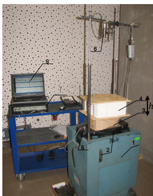
Fig. 3. General view of the shock load testing stand: 1 – shock generator; 2 – steel plate; 3 – sample; 4 – loading mass m ; 5 – shock sensors; 6 – ultrasound distance sensor; 7 – oscilloscope; 8 – personal computer, h – move direction of mass m
