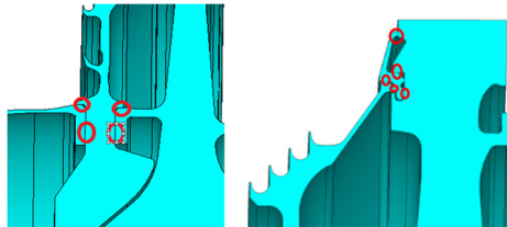
Fig. 5. Nine contact pairs on the O.S.
