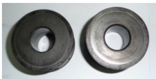
Fig. 2. Graphite aerostatic radial and axial hybrid bearing
