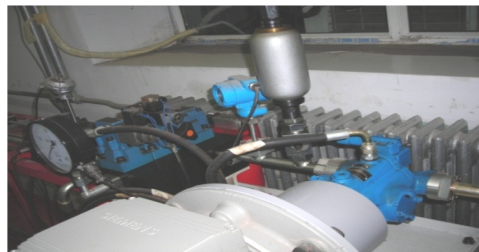
Figure 2. Test plunger pump rig.
