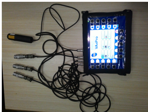
Fig. 2. Photograph of FFT analyzer
