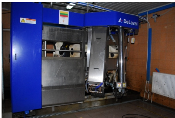
Fig. 1. DeLaval automatic voluntary milking system
