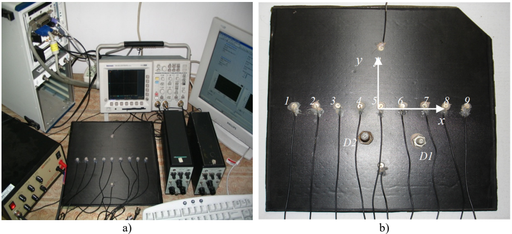
Fig. 1. a) An experimental built-in damage detection and identification system, b) a T300/648 symmetric laminate for NDT
