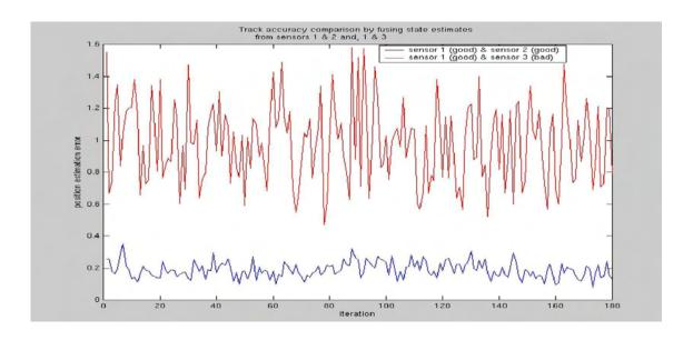
Figure 18.5: Track accuracy comparison - Noise level at sensor 1 and  $2=10\mathrm{dB}$  and at sensor  $3=0\mathrm{dB}$
