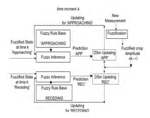
Figure 13.1: Block diagram of target's behavior tracking system
