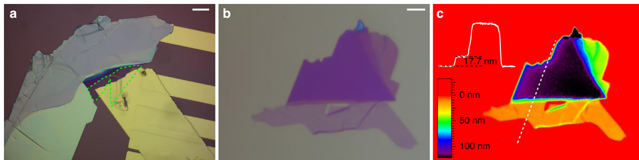
Fig. 2 Fabrication. a Microscopic image of a MoS 2 field-effect transistor device under \times 500 magnification. The monolayer is framed within the green dashed line. b, c Microscopic and phase-shift interferometric images of the WS 2 monolayer presented in the main text. The inset in c shows the optical path length difference (OPD) along the white dashed line. The monolayer has an OPD of 17.7 nm, which corresponds to a physical thickness of 0.66 nm. The scale bars in a, b are 20 and 5 \mu\text{m} , respectively
