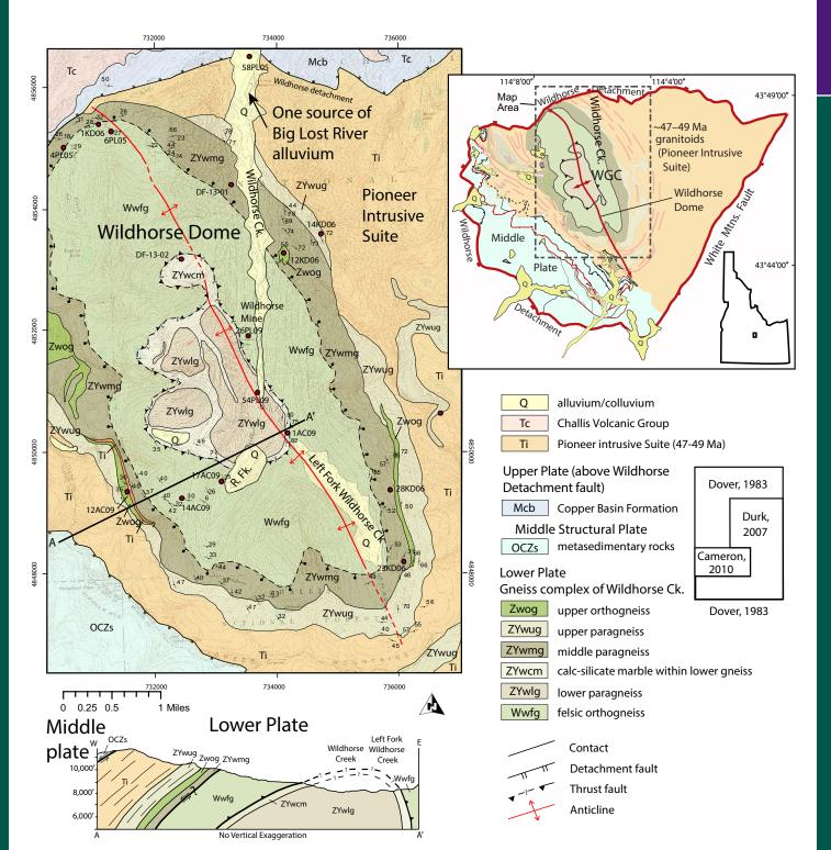
Figure 2. Geologic map and cross section of the gneiss complex of Wildhorse Creek, showing locations of samples discussed in this paper. Inset map shows regional context of Pioneer Mountain core complex (PMCC). Cross section shows structural arrangement of map units, and serves also as a stratigraphic diagram. WGC-Wildhorse Gneiss Complex.
