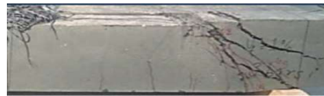
Fig. 7 Failure patterns of reinforced UHPFRC beams with a/d=1.8 : simulated (left) and tested (right)
