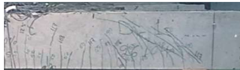
Fig. 8 Failure patterns of reinforced UHPFRC beams with a/d=2.6 : simulated (left) and tested (right)
