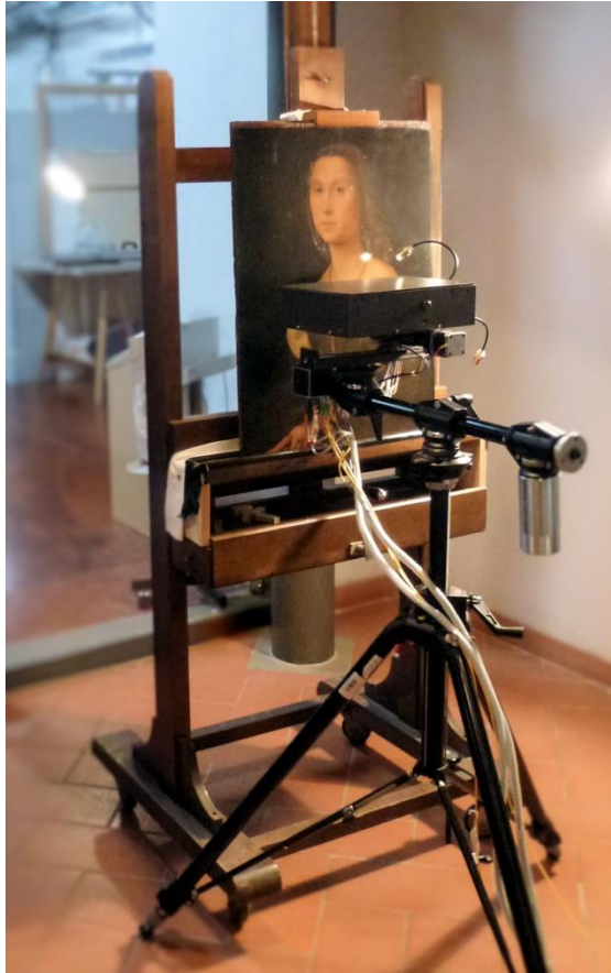
Figure 1. Examination of Raphael's La Muta with Optical coherence tomography (OCT) in Opificio delle Pietre Dure in Florence
