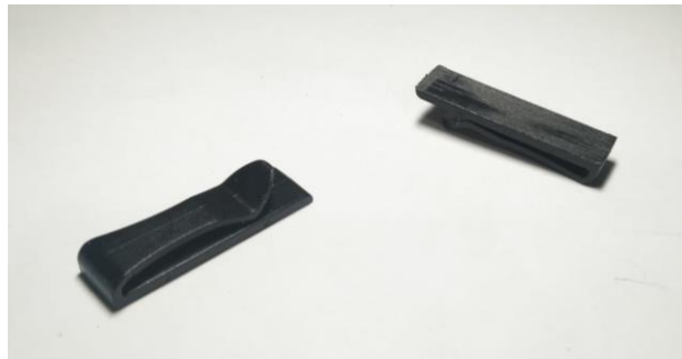
Figure 31. Buckle Webbing Ending Clip cut and sanded.
