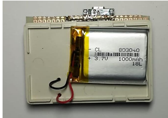
Figure 34. Lithium battery glued to the shield cover.
