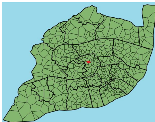
Figure 17: Assumed location of a subscriber based on its call detail record (reded polygon)
