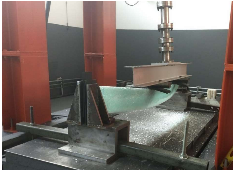
Figure 5.18 – First Beam Prototype Rupture. Source: Author (2019).
