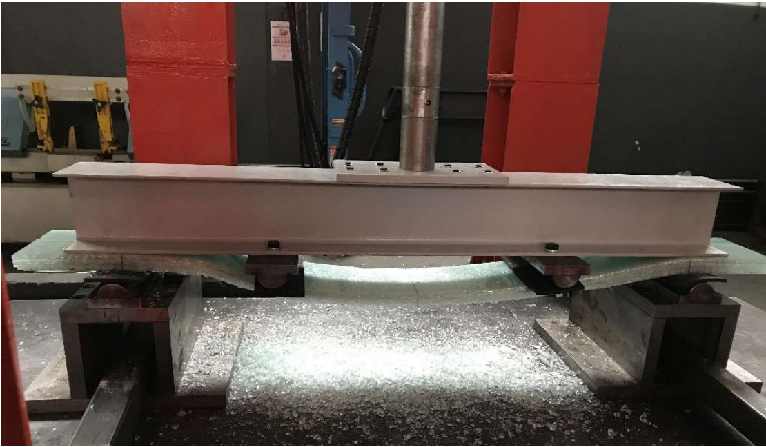
Figure 5.4 – First Slab Prototype Rupture. Source: Author (2019).
