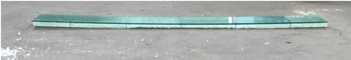
Figure 5.13 – Third slab prototype after rupture and load removal. Source: Author (2019).
