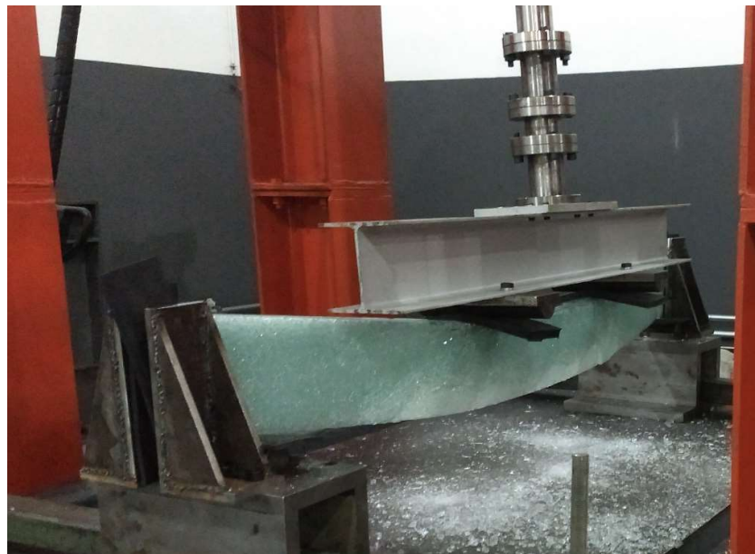
Figure 5.22 – Second Beam Prototype Rupture. Source: Author (2019).
