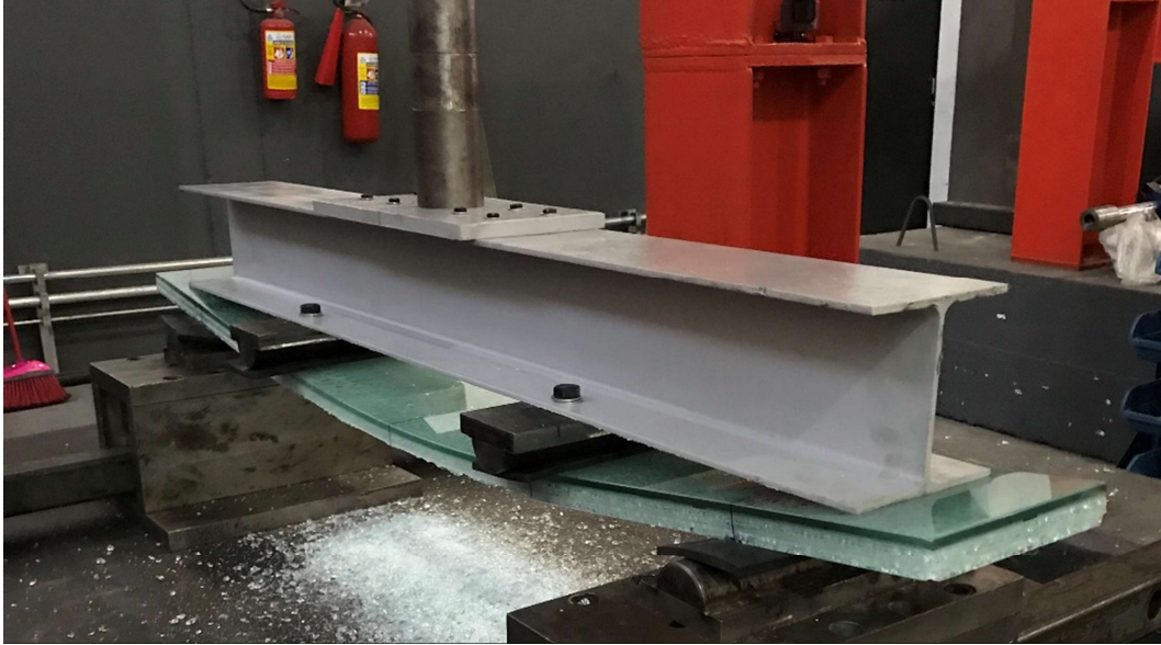
Figure 5.12 – Third Slab Prototype Rupture. Source: Author (2019).
