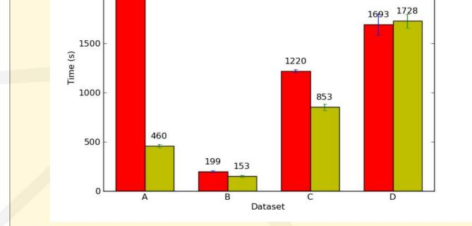
For very large files the performance is similar to the old system, but as file sizes decrease the physical transfer becomes a smaller part of the whole process. The new framework greatly reduces staging time in these cases by separating physical transfer from other operations.
