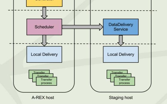
To increase network throughput, extra staging hosts running a **Data Delivery Service** can be added to the system to which physical transfers can be off-loaded.
