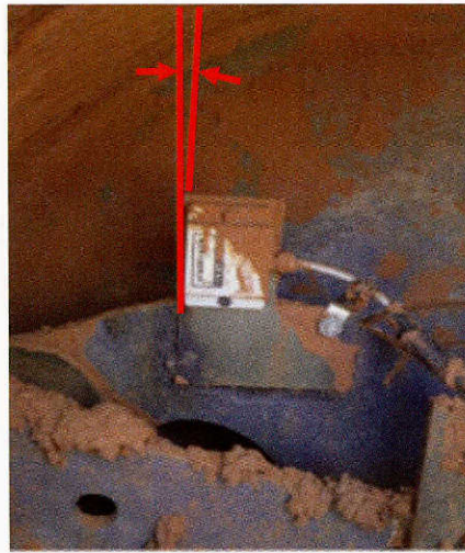
Figure 5.1 – Non-Vertical Mounting of Retrofit Accelerometer.
