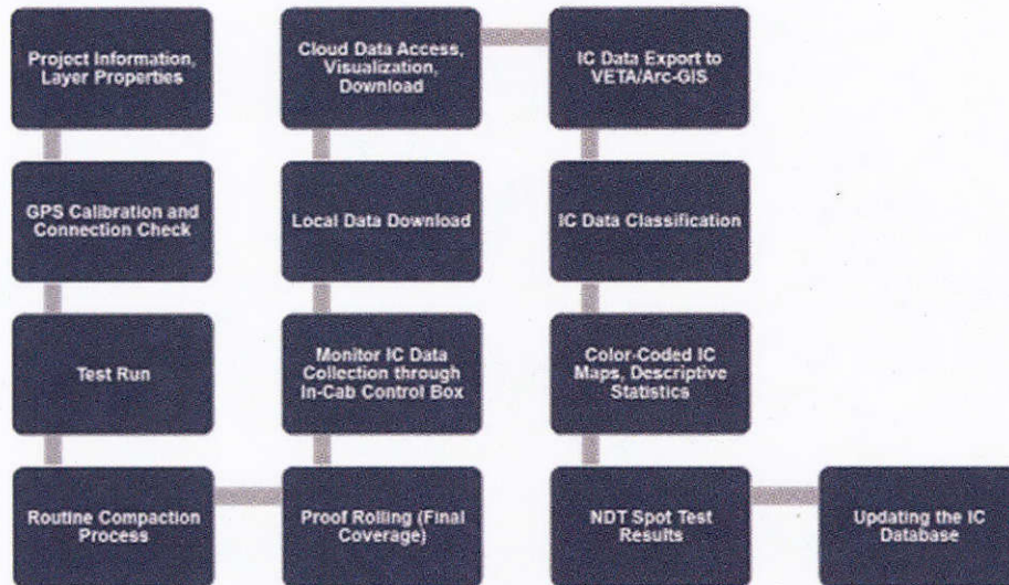
Figure 4.1 – Flowchart of Collecting and Preparing IC Data to Update the IC Database.
