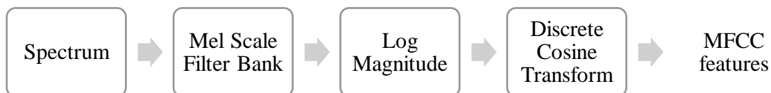
Figure 2.10 - Process of obtaining the MFCC features (Adapted from [21])
