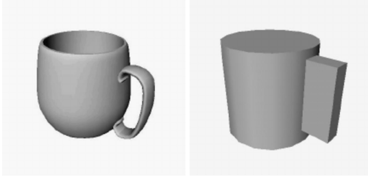
Figure 2.3: Approximation of a mug to a cylinder and a box [MKCA03]
