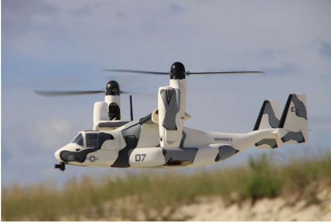
Figure 1.4 – Rotormast UAV tiltrotor modeled after the Bell Boeing V-22 Osprey 5
