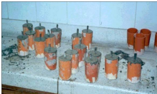
Figure 2. Reinforced concrete specimens
