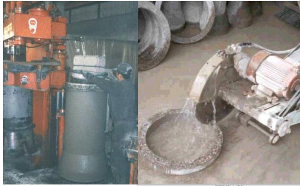
Figure 1. Preparation of plain concrete specimens
