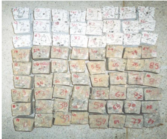
Figure 4. All samples after the second week of sulphuric acid contact
