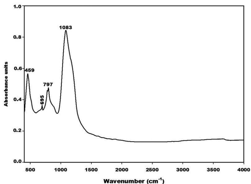
**Figure 4.** Infrared spectra of metakaolin (MK-Dib<sub>0</sub>).
