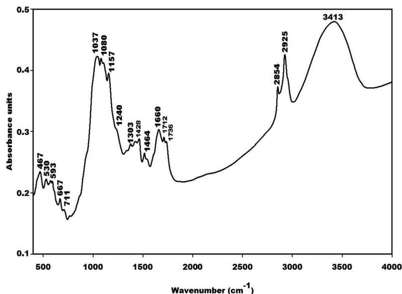
Figure 5. Infrared spectra of rice husk (RH).
