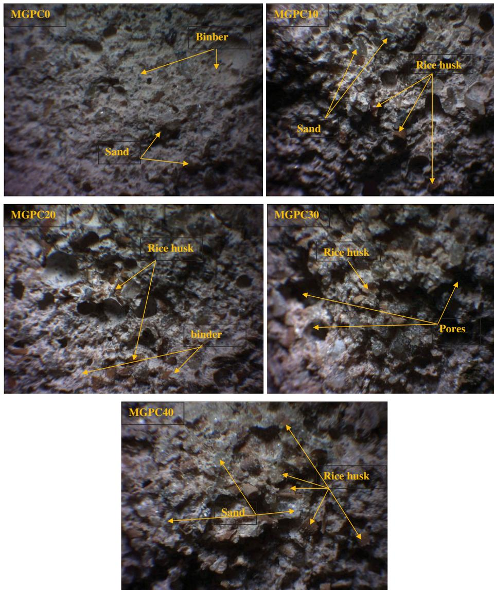
Figure 12. Optical microscope images of geopolymer mortars.
