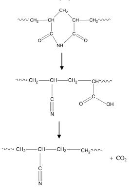
With the formation of pores through the polymer degradation in ceramic bodies characterized by the releasing of  $NH_3$  and  $CO_2$  gases then assumed that the number of moles of polymer in the ceramic body will affect the density of ceramics. The parameters that were examined which is the ratio of monomer and crosslinker. The hardness of porous ceramic body are shown in Table 1.
