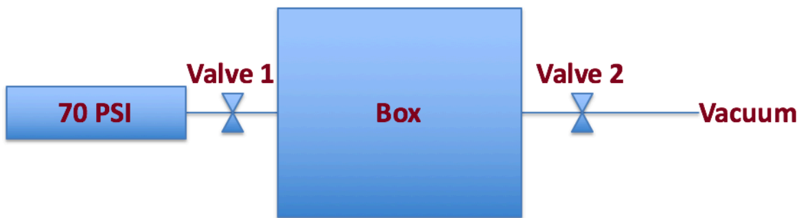
Figure 2: Schematic of the DPBLD. Valve 1 opens to increase the pressure to the desired maximum pressure. Valve 1 closes, and simultaneously, valve 2 opens to decrease the pressure back to a normal IAP. Once a normal IAP is reached, valve 2 closes. Valve 1 and valve 2 are both Arduino controlled solenoid valves.
