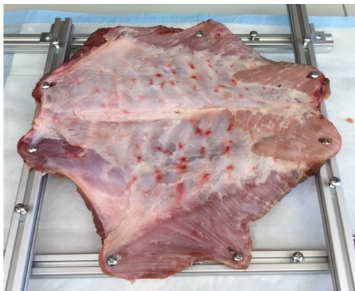
3: The tissue sample is mounted on the posts of the aluminum frame via holes created with a biopsy punch
