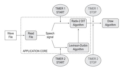
**Figure 6**. Timers position diagram. Timer 1 measures the response time of the spectral data calculation. Timer 2 measures the response time of the envelope data calculation
