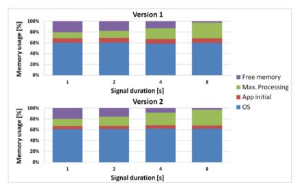
**Figure 8**. Memory footprint measurement. Operating system requires around 60% of memory space, while the spectral calculation requires between 10% and 30% of memory space
