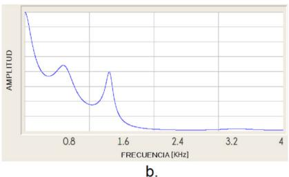
Figure 4. Spectrum of speech signal mamá (mom) and its LPC model. a) spectrum of the signal. b) Spectrum of the LPC model
