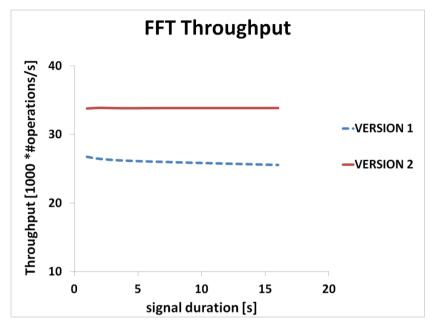
**Figure 9**. Throughput measurement. The throughput of version 1 (spectral analysis) of the application decreases when signal duration increases, while the throughput of version 2 (spectrographic analysis) of the application is constant, regardless of the signal duration
