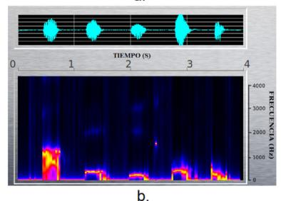
**Figure 5**. Spectrogram of speech signal "a-e-i-o-u" (pronounced in spanish) and its LPC model. a) Spectrogram of the signal. b) Spectrogram of the LPC model
