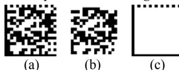
Gambar 1. Struktur Data Matrix : (a) data matrix bar code, (b) data region, (c) pola finder
