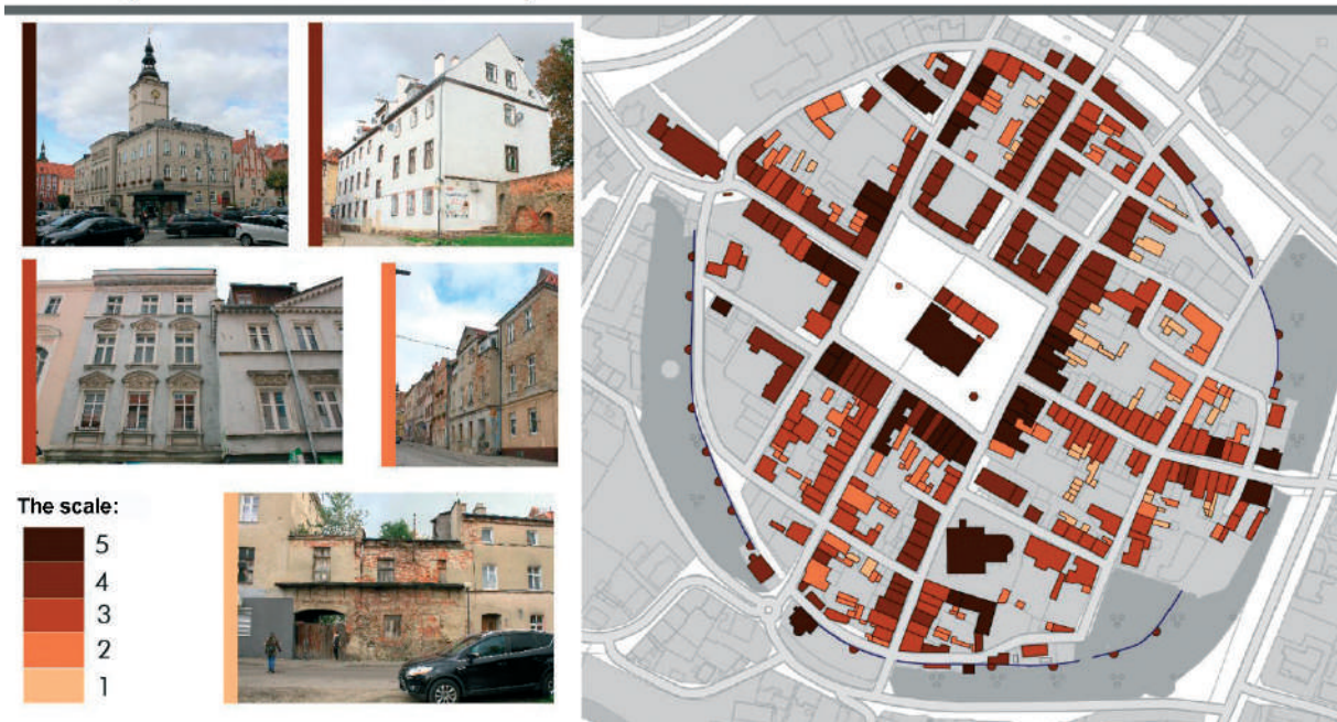
Figure 4. Analysis of the landscape – technical condition. (authors: Katarzyna Kraśnicka, Marta Jastrzębska, Dominika Koncewicz 2017/2018). Depiction of the scale: 1–6 from the lowest to the highest values
