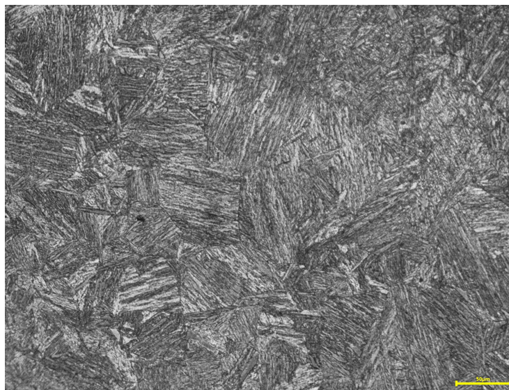
Fig. 5. Microstructure of the weld (joint cross-section with the use of micro-jet cooling); the scalebar is 50 \mu\text{m} .
