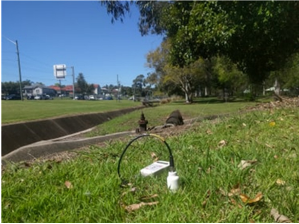
Figure 2: Theta Probe used for soil moisture measurements along the transect.
