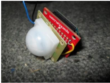
Fig. 6. PIR sensors monitors the movement across the room
