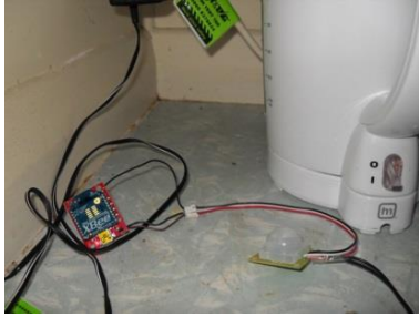
Fig. 5 Sensor used to monitor the usage of electrical devices
